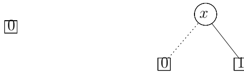
Figure 6.6. The BDDs (a) B_0 , representing the constant 0 boolean function; similarly, the BDD B_1 has only one node 1 and represents the constant 1 boolean function; and (b) B_x , representing the boolean variable x .
